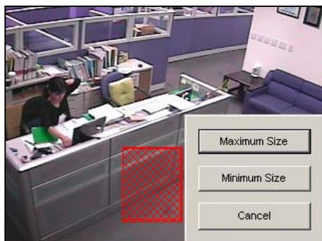
**Figure 1-63** Defining the min. and max. detection size
