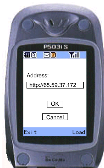
Figure 6-66 Entering the IP address of GV-server
