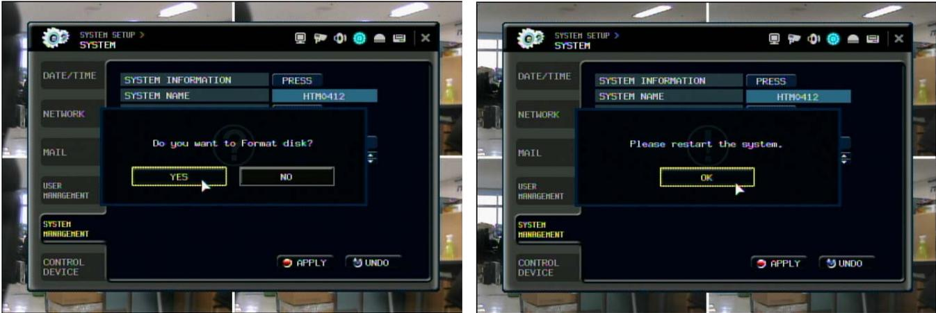
**SYSTEM DATA** : System settings can be saved to a USB memory stick. The settings can be reloaded in case of accidental factory reset or can be transferred to another DVR if multiple units need to be installed with the same settings.
