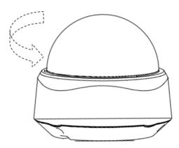
Figure 2.3 Remove the Bubble
