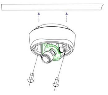
Figure 2.4 Secure Back Box to the Wall
