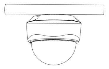
Figure 2.6 Replace the Bubble
