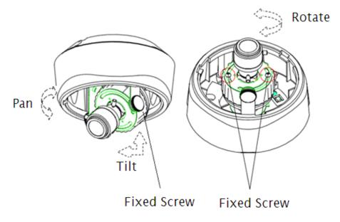
Figure 2.5 Adjust Lens
