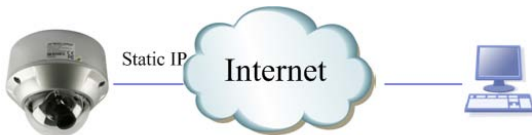
Fig.3.5.2 Static IP access IPC directly
