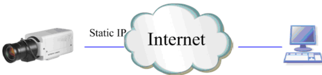
Fig.3.6.2 Static IP access IPC directly
