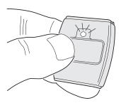
PROGRAM THE TRANSMITTER INTO THE RECEIVER BY PLACING THE RECEIVER INTO PROGRAM MODE. THEN SEND A SIGNAL TO THE RECEIVER FROM THE TRANSMITTER. REFER TO THE RECEIVER'S PROGRAMMING INSTRUCTIONS FOR DETAILS.
