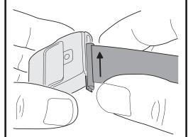
NOTE: THE END OF STRAP WITH VELCRO ATTACHES TO THE END CLOSEST TO THE SIGNAL INDICATOR
