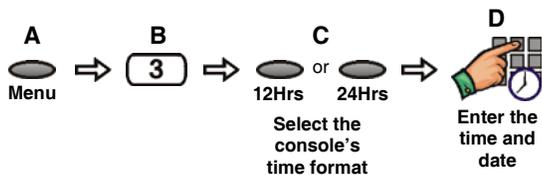
A- Press the **[MENU]** action key (the right action key located under the right side of the LCD screen).
